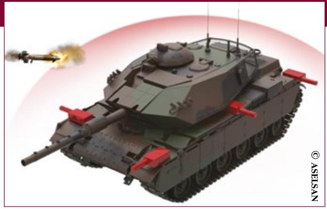
The M60 tank is integrated with six PULAT active protection system countermeasure modules.
