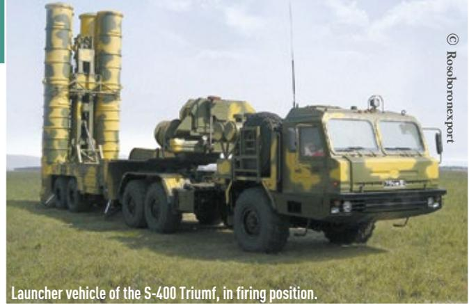
Launcher vehicle of the S-400 Triumpf, in firing position.
